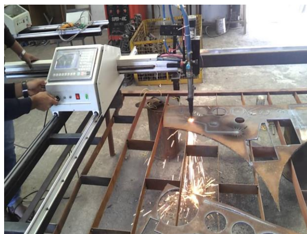
Fig. 3 - Profile Cutting With A CNC Machine [9]
