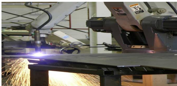
Fig. 2 - Profile Cutting Performed by an Industrial Robot [5]
