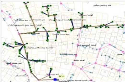
Fig. 2: Feeder single line in GIS (First study)
