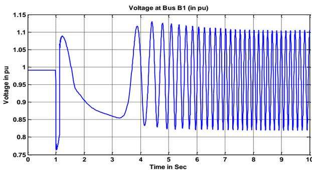
Fig.5 Voltage at Bus\_1 without PSS.
