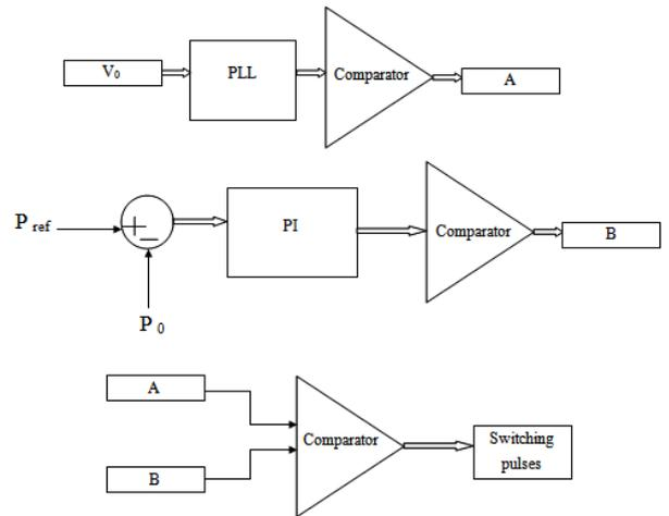
Fig. 3.4 Closed loop configuration of PDM scheme
