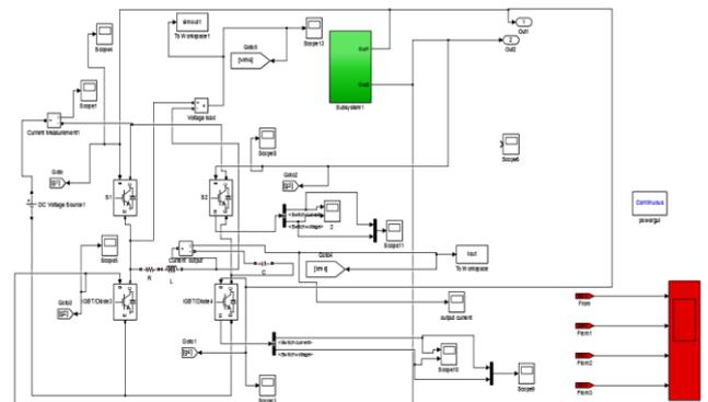
Fig.4.1 Simulink diagram of a FB topology using PDM
