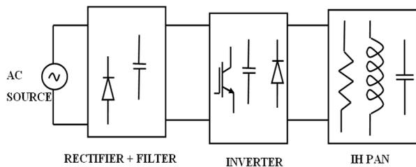
Fig. 1.1 Arrangement of an induction heating system
