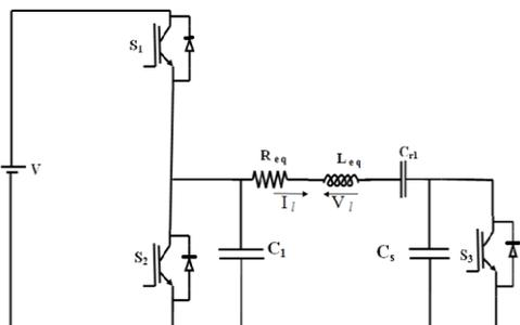
Fig. 2.4 The asymmetrical configuration of IH topology
