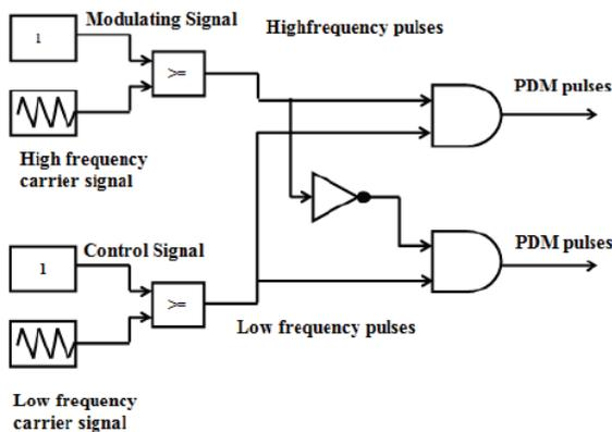
Fig.3.3 Logic circuit for PDM signals
