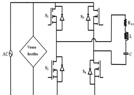
Fig. 2.5 The Vienna rectifier configuration
