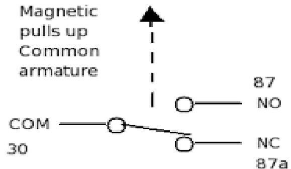
Fig.2- NO NC contact of electromagnetic relay
