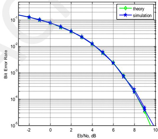
Figure 13: curve of Gaussian noise BER for wavelet source coding with OFDM
