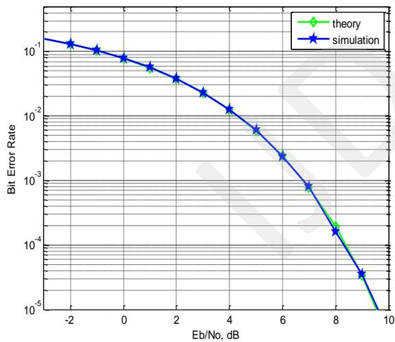
Figure 5: curve of Gaussian noise BER for DCT source coding with OFDM
