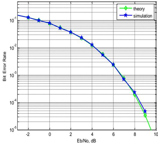
Figure 9: curve of Gaussian noise BER for wavelet source coding with OFDM
