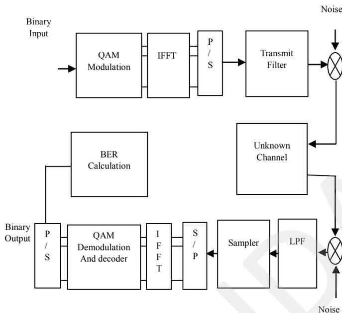
Fig.1: block diagram of OFDM
