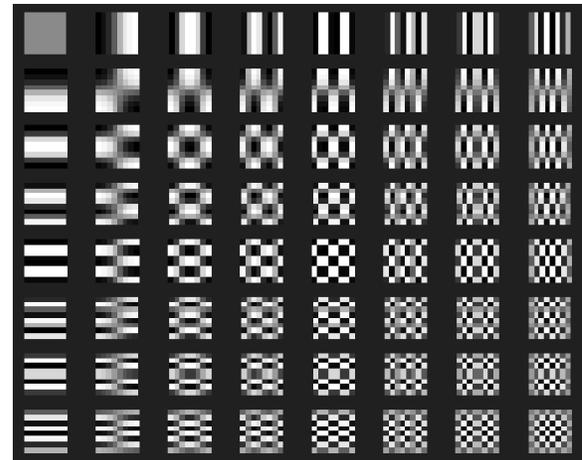
Figure 2. Two dimensional DCT basis functions ( $N = 8$ ). Neutral gray represents zero, white represents positive amplitudes, and black represents negative amplitude [10].
