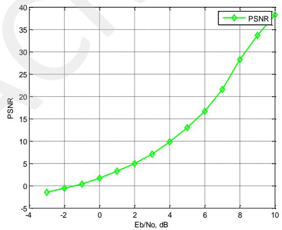
Figure 7: PSNR curve for DCT source coding with OFDM
