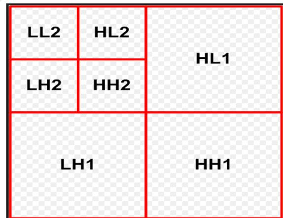
Fig.4: Pyramidal structure
