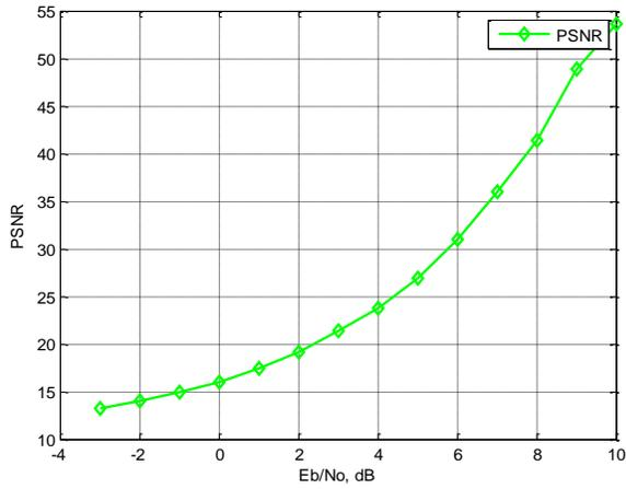
Figure 15: PSNR curve for FFT source coding with OFDM
