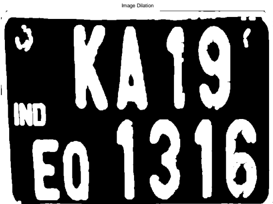
Figure 4.7: Perform morphological dilation with disk structure of radius 5 pixel
