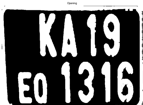
Figure 4.8: Perform morphological opening, remove white areas less than 40000 sq. pixel
