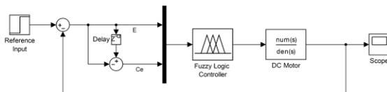
Figure 5: Simulink model for DC Motor controlled by Fuzzy Logic controller
