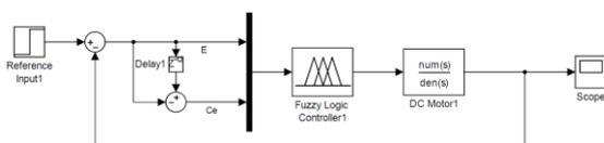
Figure 6: Simulink model for DC Motor controlled by Neuro-Fuzzy controller
