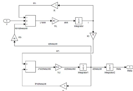
Figure 1: Simulink model for brushless DC motor
