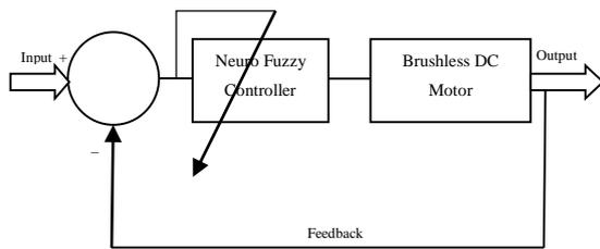
Figure 3: Basic block diagram for proposed Neuro fuzzy controller based BLDC motor speed control system
