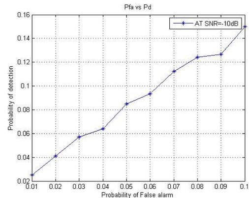
Figure 3: Probability of false alarm V/S probability of detection at SNR= -10 dB
