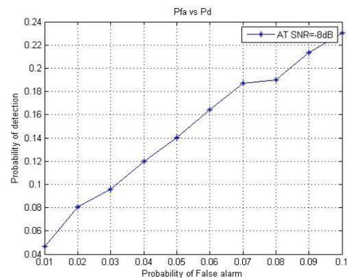
Figure 4: Probability of false alarm V/S probability of detection at SNR=-8 dB
