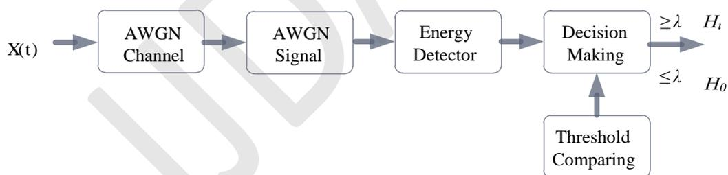
Figure 2: A Block Diagram of the Energy Detection [10]
