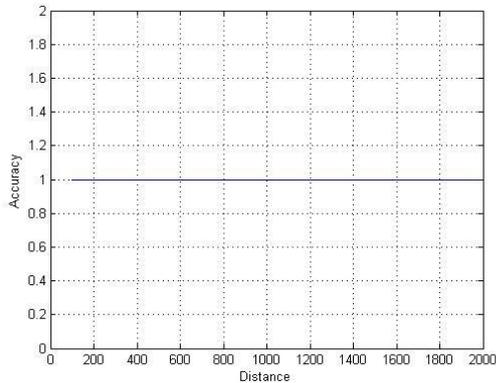
Figure 11: Distance V/S accuracy curve for soft decision spectrum sensing
