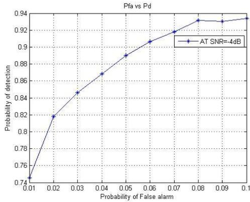
Figure 6: Probability of false alarm V/S probability of detection at SNR=-4 dB
