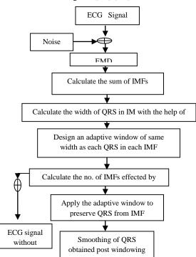
Figure 1: Block diagram of modified EMD based algorithm for denoising of the ECG signal
