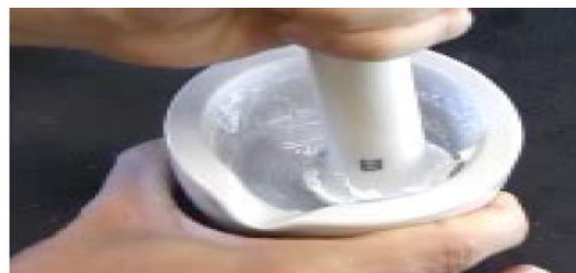
Fig. 4 Grind of nanocrystalline titanium dioxide in a mortar and pestle & A few drops of Triton X-100 surfactant.
