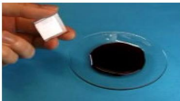
Fig. 10 Immerse the coating in a source of anthocyanins such as pomegranate
