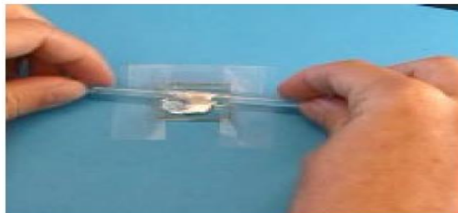
Fig. 7 The titanium dioxide paste and spread using a glass rod
