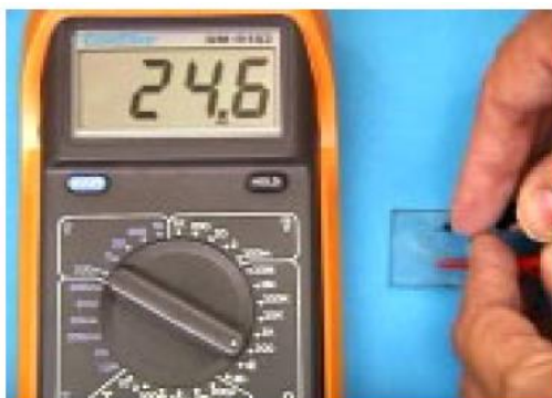
Fig 5 Identify the conducting side of glasses
