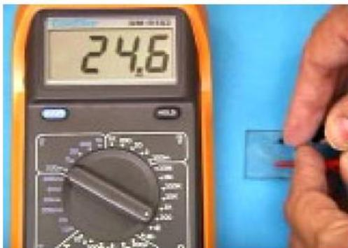
Fig 5 Identify the conducting side of glasses
